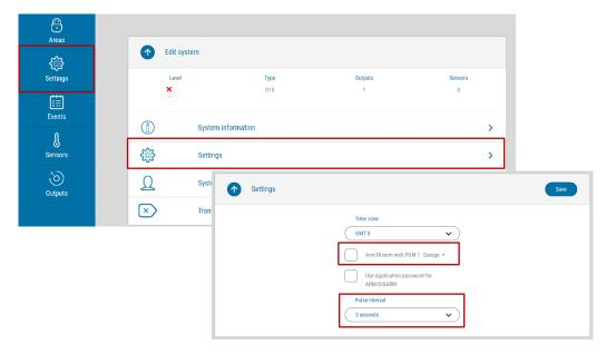
**IMPORTANT!** In Protegus app one PGM output can be assigned to control one Area (1 PGM - 1 Area; 2 PGM - 2 Areas) regardless of how many areas are controlled by same keyswitch zone in panel.
